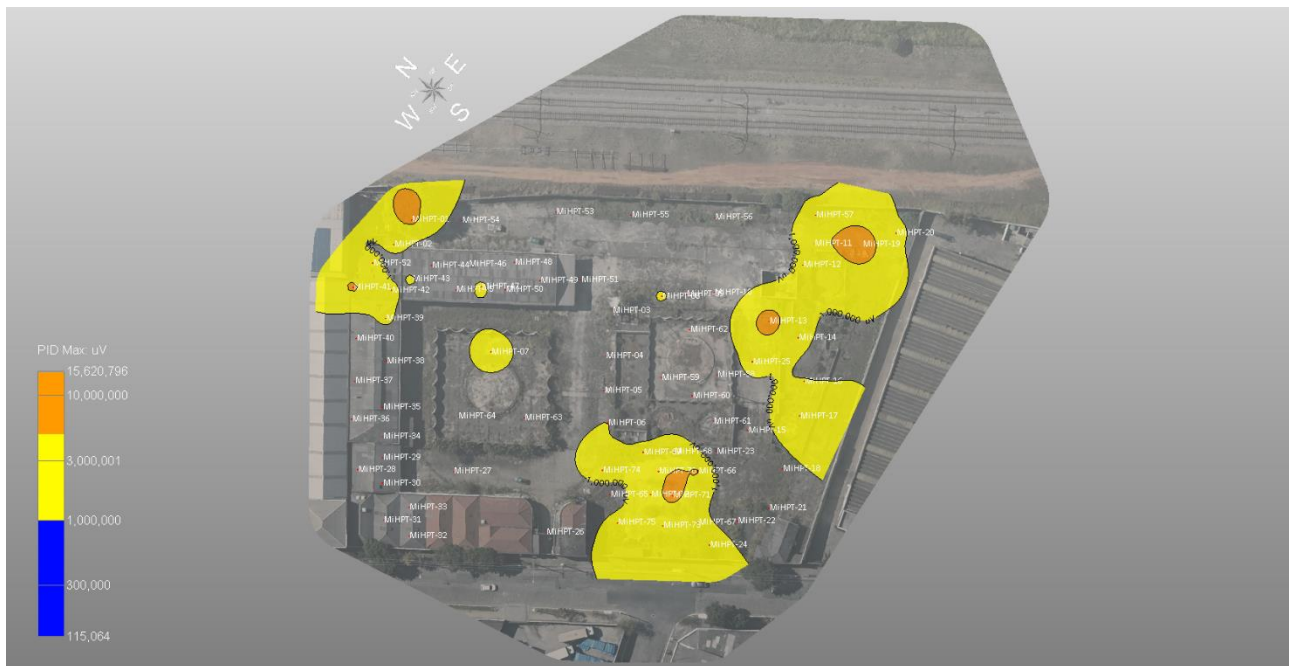
Picture 1: Areas with higher readings from the PID sensor of the MiHPT system identified source zones of hydrocarbon contamination and its correct extension.
