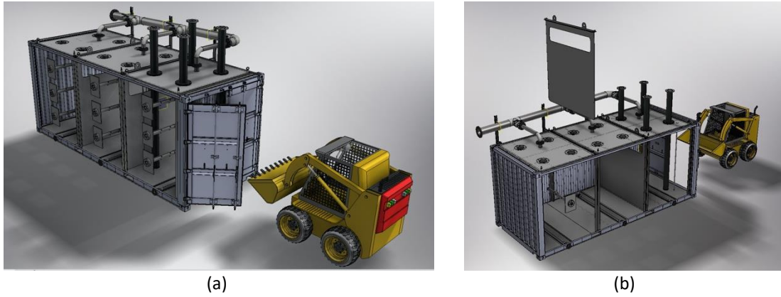
Figure 2 – (a) Details of the test cell design complete assembly, (b) detail of the removable metal sheet that separate the chambers
